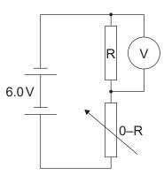
What are the initial and final voltmeter readings when the variable resistor is increased from an initial resistance of zero to a final resistance of R?
