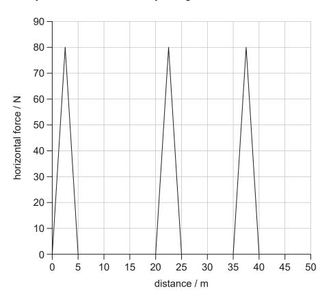
A constant frictional force of 2.0 N opposes the motion. What is the final kinetic energy of the object after it has moved 50 m?
